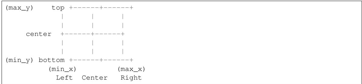
Alignment options are given as – separated tuple, allowing for combinations of left, center, right with bottom, center, top.
